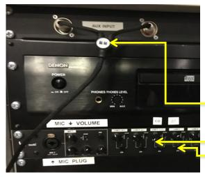
3.To play an Auxiliary (AUX) Device e.g. Smart Phone, iPod or sound via a Laptop or TV, press the small on/off button on the control panel marked "AUX" – a green indicator light comes on.
